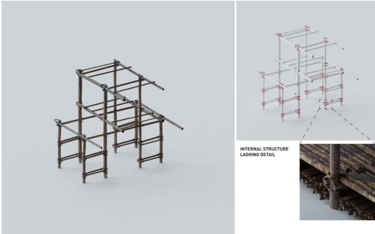
Fig. 8: Detail showing the lashing of the structure in the Rhinoceros 3D model
