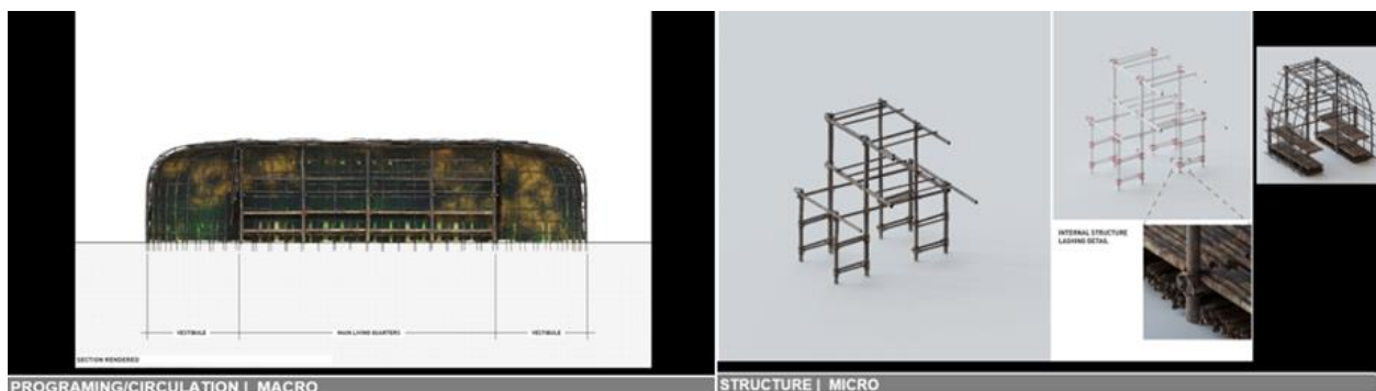
Fig. 7: Textured section drawing of a longhouse to showcase the circulation and organization of space (Left). Isometric views of the longhouse fragment highlighting details such as the lashings (Right)
