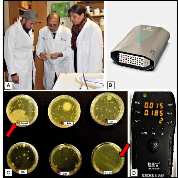
Fig. 3A. Examining the Petriplates. B. AFL Mini Sanifier II<sup>®</sup>. C. Petriplates showing gradual reduction of the microbial colonies on running the AFL Mini air purifier. D. Final counts of Formaldehyde, Total VOC and PM2.5 using a Garosa Air Quality Monitor Formaldehyde Detector and Accurate PM2.5 Micron Particulate Matter Dust Pollution Multi Tester.
