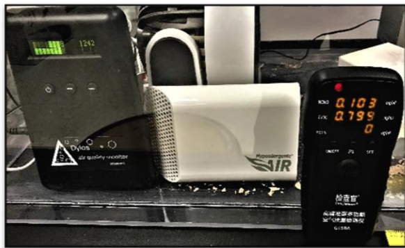
Fig. 3. Testing the Mold Guard unit in the AO fiberglass chamber.
