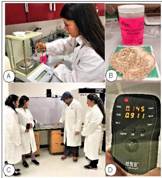
Fig.4. Steps of testing the Mold Guard unit: A. Weighing the Particulate Matter. B. PM 2.5 testing Dust. C. Uniform spreading of the Particulate Matter in the AO Fiberglass chamber. D. Meter readings.
