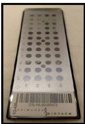
Figure 1. Fleximass Polymeric Sample Plate. Rows B and J show recently deposited microbial samples combined with CHCA matrix. The three sample wells between columns 2 and 3 are for the DH5 \alpha -E TM standard.
